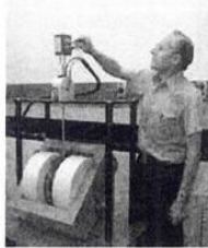
Bob Thurber connecting cables to the sample holder for a Hall effect measurement.
